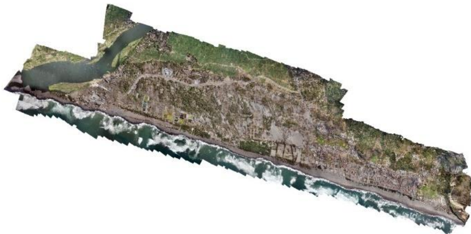
Figure 8. Small format aerial photo derived from UAV acquisition after the mosaic process
