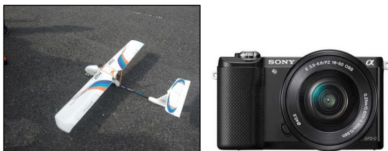
Figure 2. Sky Walker fixed-wing (left) as a platform and Sony A5000 camera (right) as payload
