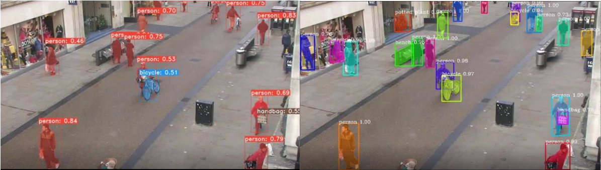
Figure 3 Town Centre video sample frame Right Yolact ++ result, Left Mask-R CNN result
