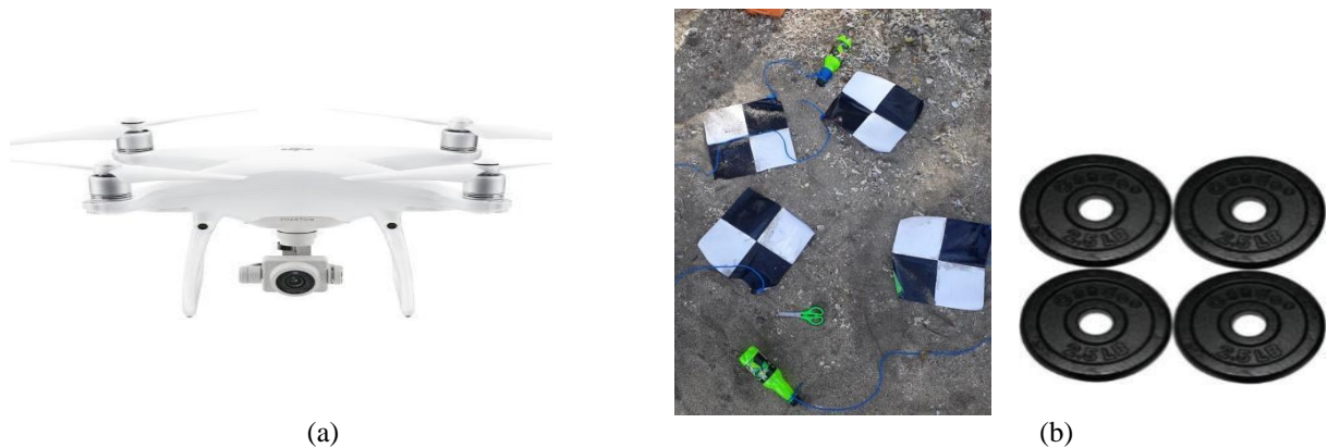
Figure 3. Imaging sensor (a) and materials in creating grid targets (b) in aerial mapping
