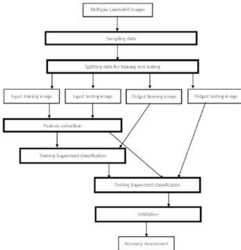
Figure 1 The flowchart of our methods to obtain the accuracies of land cover classification methods.
