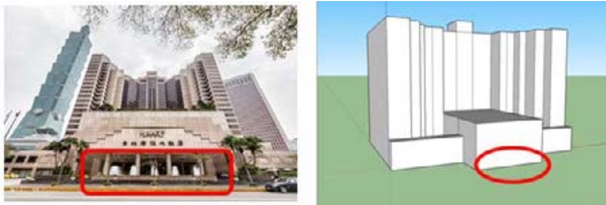
Fig. 1. Arcades or open spaces on first floors resulting insignificant discrepancies between the reality (left) and the generated CityGML LOD-1 building model (right)
