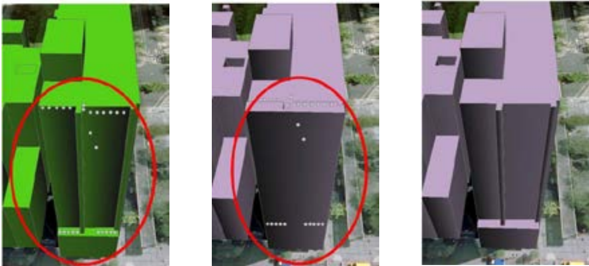
(c) insufficient LiDAR point clouds for construction of the small objects (left: reference data; middle: the constructed model based on the point clouds; right: adjust the constructed model manually)
