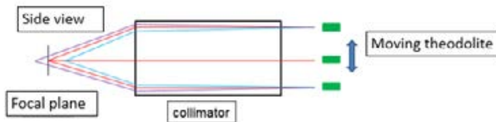
Figure 3. Schematic diagram of the collimation measurement in vertical direction.
