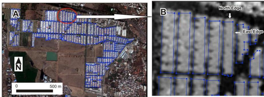
Figure3. Preparation of reference data: (A) Building polygons are digitized on top of multispectral image; (B) Digitization of each block as single polygon
