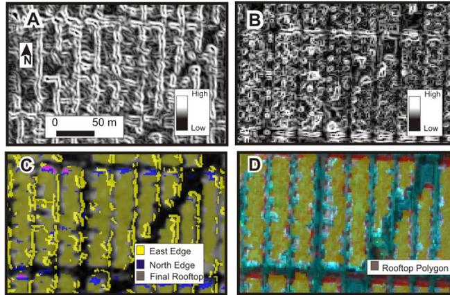
Figure 4. automated extraction of building polygons, A. East edge derived from Relief shaded image, B. North Edge derived from Near Infrared Band C. North Edge and East Edge classes, Building polygons are extracted in relation to Edges D. Individual polygon for each block
