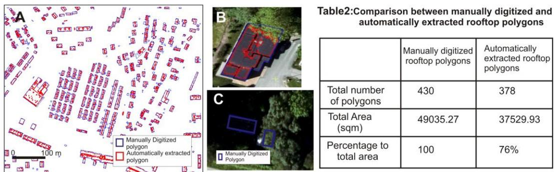
Figure 9. A. Visual comparison between automated and manually extracted rooftop polygons, B & C. Automated method did not extract the roofs which are covered with vegetation.
