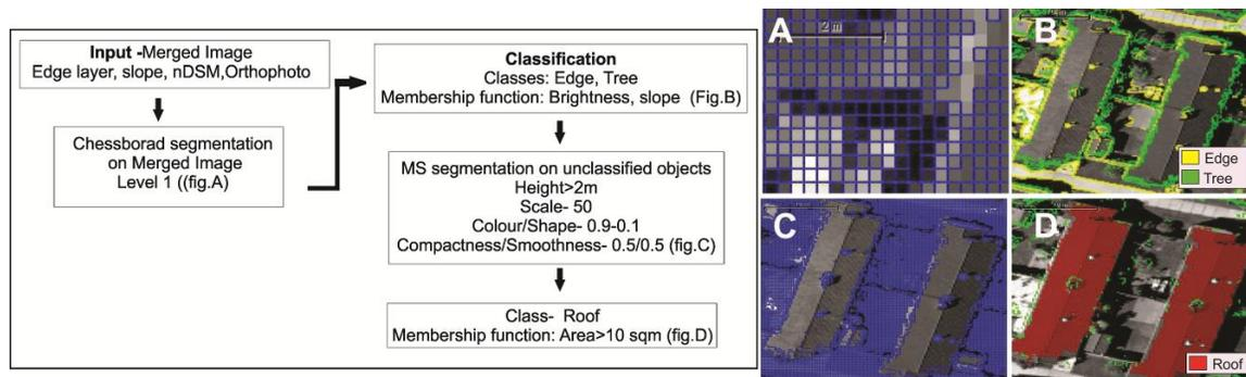
Figure 7. Flow chart describes automated extraction of roof area (see text for detail) with images showing intermediate outputs.
