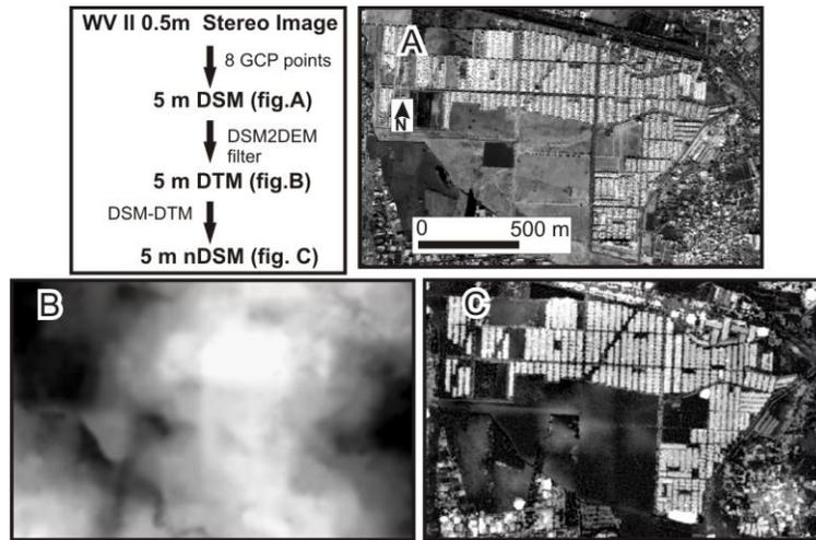
Figure2. Flow chart describes image preprocessing with images showing intermediate outputs.
