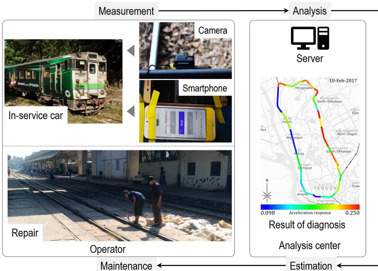
**Figure 3.** The overview of the portable monitoring system and flow of maintenance. Smartphone based accelerometer measures car-body acceleration, and the data is analyzed and diagnosed. If track irregularity is estimated, operator repairs a damaged track based on a result of diagnosis.
