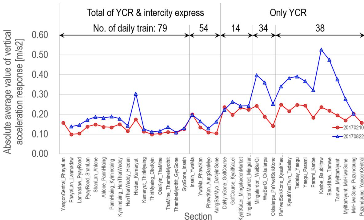
**Figure 4.** Car-body vertical acceleration response for each section separated by stations based on measurement data obtained on 10 February 2017 (red line) and on 22 August 2017 (blue line). The section of left from Danyingone Station is run by circular train, intercity express, suburb train and local section train. The section of right from Danyingone Station is the section run by only circular train.
