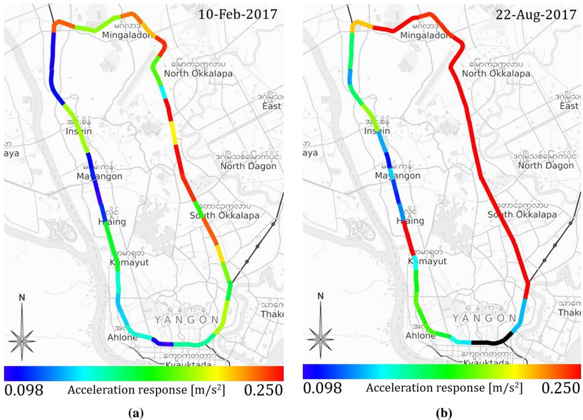
**Figure 5.** Condition mapping based on analysis of car-body vertical acceleration response for each section separated by 38 stations; (a) Result from measurement data on 10 February 2017, (b) Result from measurement data on 22 August 2017.
