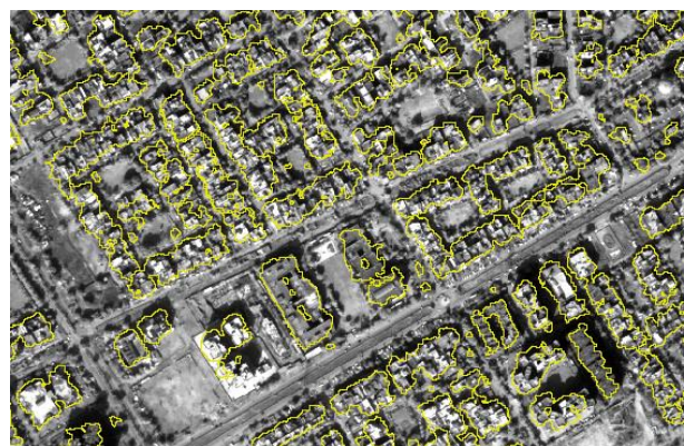
Figure 8: Building Footprint extracted from Pleiades data overlaid on Kompsat-3 Ortho, Part of Delhi NCR
