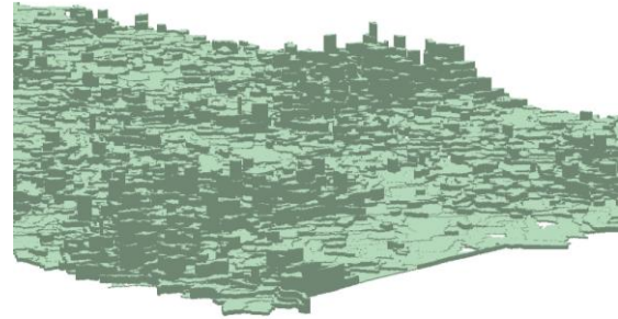
Figure 10: 3D view of Building Footprint extracted (Kompsat-3 Data), Part of Delhi NCR
