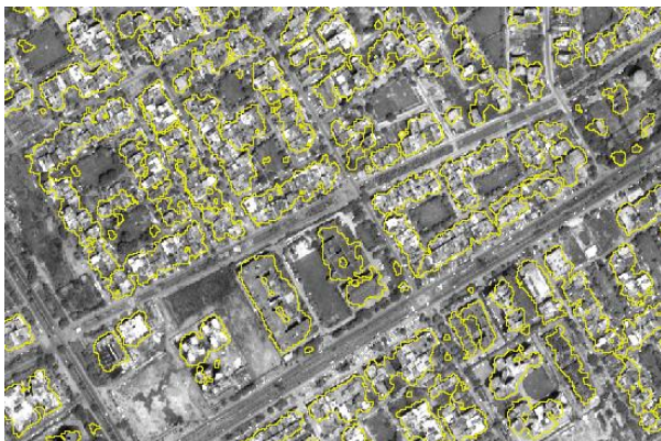
Figure 7: Building Footprint extracted from Pleiades data overlaid on Pleiades Ortho, Part of Delhi NCR
