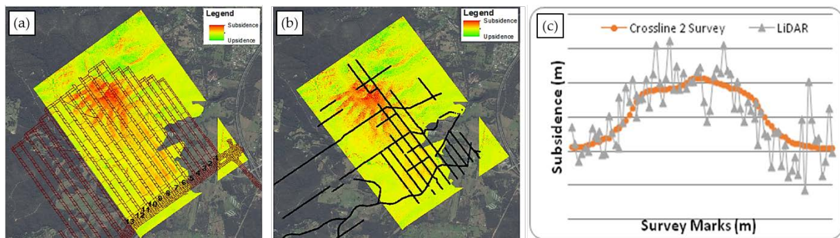
Figure 8 Overlay of subsidence derived from LiDAR on (a) underground longwall panels and (b) survey lines and (c) comparison of LiDAR measurements against a crossline survey line measurement
