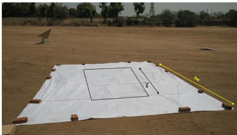
Figure 3: Sampling plan for the measurements (measurements were confined to inner 3m \times 3m)
