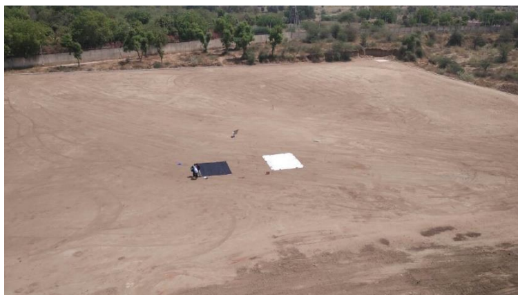
Figure 2: Artificial targets deployed at SAC-Bopal calibration site
