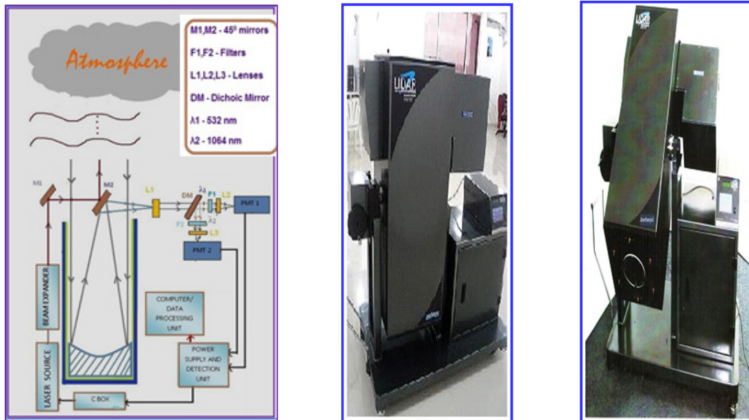
Figure 1 The Schematic diagram and the lidar system developed
