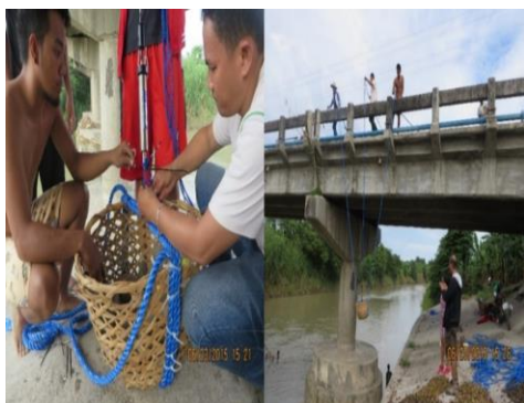
Figure 8. DCFM deployment in Lasang River at Little Panay Bridge, Panabo City, Davao del Norte.
