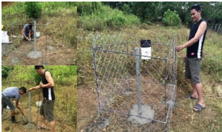
Figure 6. Installation of rain gauge station at Brgy. Tapak, Paquibato District, Davao City.
