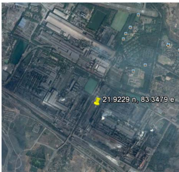
Figure 4. Jindal steel mill, detected as a persistent site with lower temperature than a gas flare. Average temperature is 1046 K.
