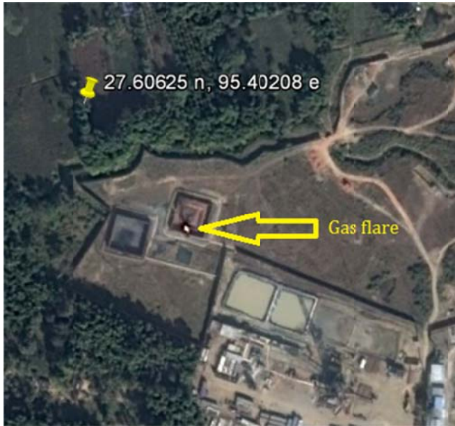
Figure 3. Gas flare detected from the persistent IR emitter set from 2015 VIIRS data. Average temperature is 1686 K. The location identified in VIIRS is 120 meters away from the actual flare.
