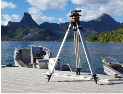
Figure 10. Leveling with green laser pointer for accurate height difference determination in control points.
