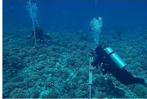
Figure 10. Leveling with green laser pointer for accurate height difference determination in control points.
