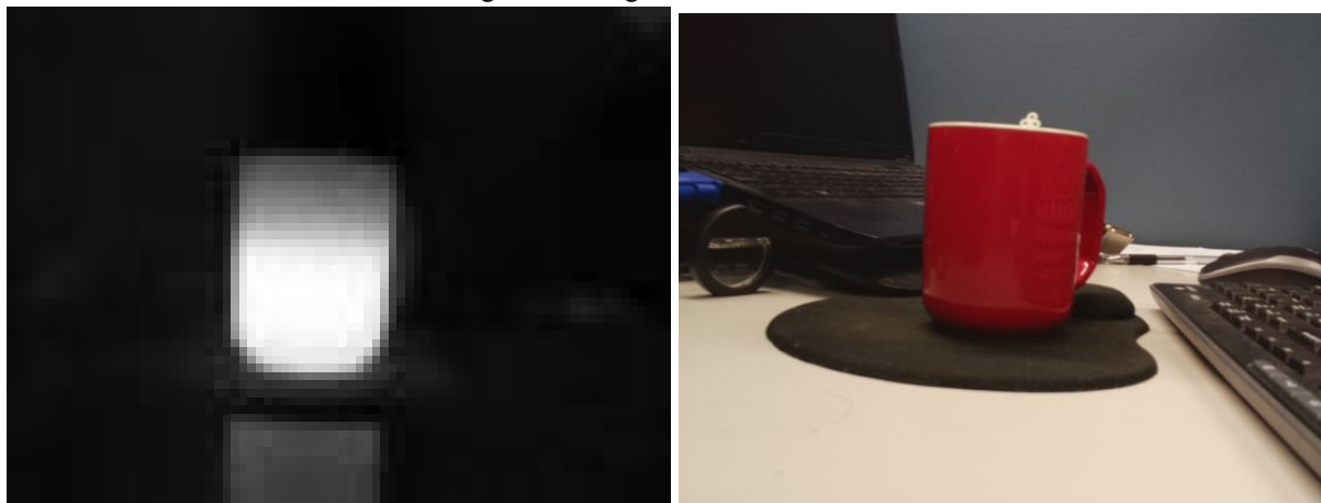
Figure 3.4 Same mug insulated on a black mattress(as a blackbody)
