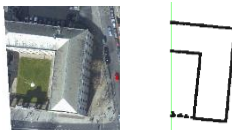
Figure 10. (a) Represents the aerial image of the partial building (b) Represents the seed points of the extracted footprint
