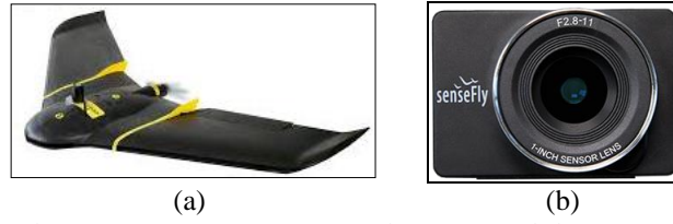
Figure 3. Research Instruments: (a)eBee senseFly Drone and (b)S.O.D.A senseFly Camera
