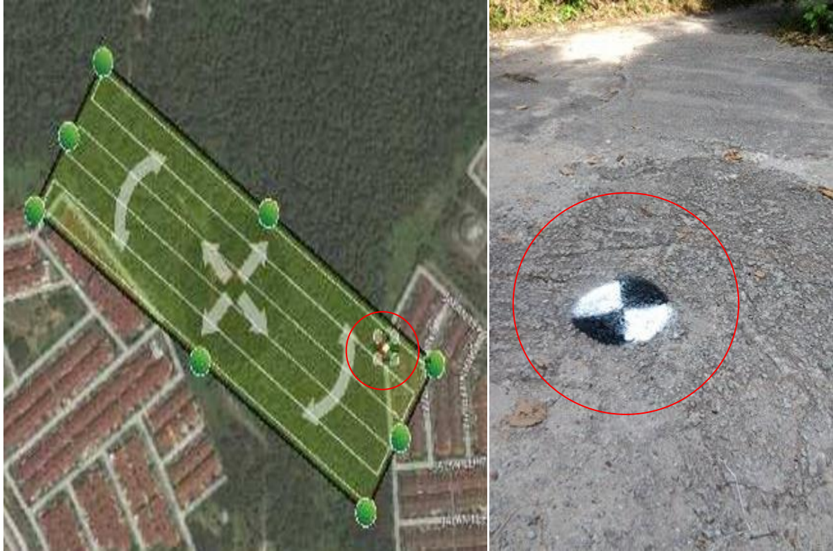
Figure Error! No text of specified style in document.. The UAV flying (left) and GCP's maker (right).
