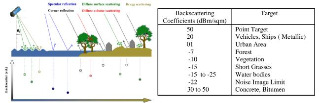
Figure 3: Radar Backscattering of radar signal
