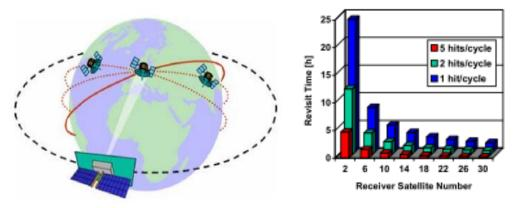
Figure 8: Frequent Monitoring with bi-static SAR satellite constellation. Left: Geostationary radar illuminator with LEO receivers. Right: Revisit times for local acquisition scenario (X-band SAR System, Transmit Power: 1KW, Transmitter antenna size: 100sqm, SAR receiver antenna size: 6sqm, SAR receiver altitude : 400Km (LEO), Ground range and azimuth resolution: 3m)
