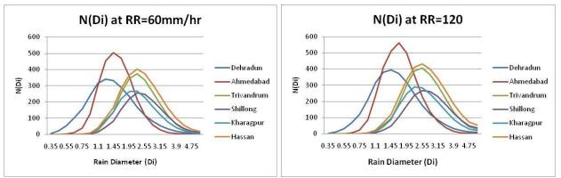
Figure 1: Variation of RDSD Spectra in different locations at 60 mm/hr rain and 120 mm/hr rain rate
