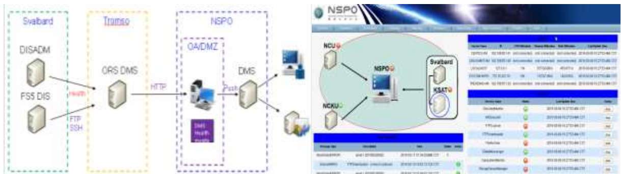
Figure 7: MMI has the capability of monitoring and remote controlling/operating ORS-DMS site
