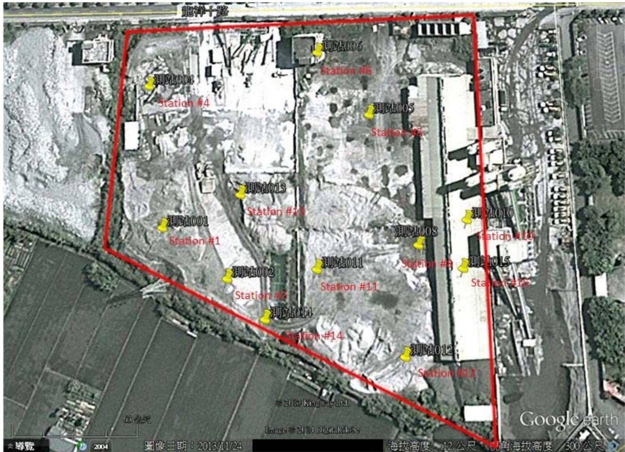
Figure 2 Locations of 12 laser scanning stations
