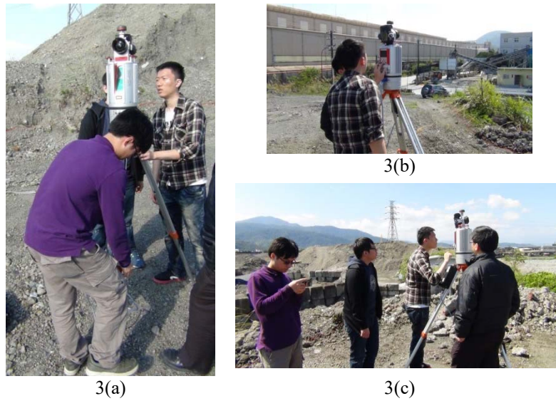
Figure 3 Pictures of field laser scanning work: (a) scanner leveling, (b) scanner set-up, (c) scanner checkup
