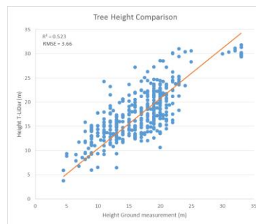
Figure 8. Comparison of tree height from field measurements and tree height derived from TLS.
