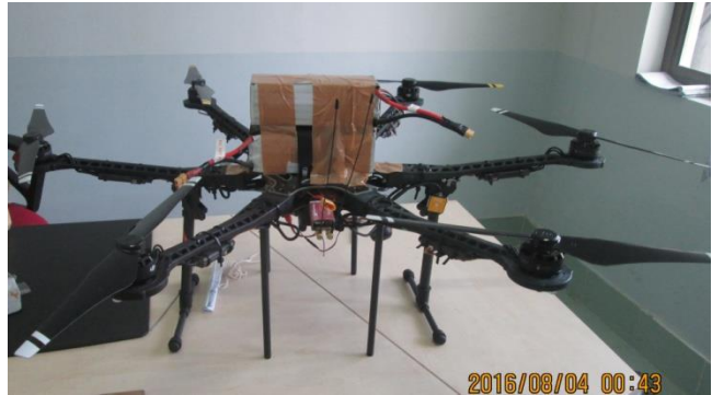
Figure 16: Hex copter with dummy payload of 1.5 kgs.
