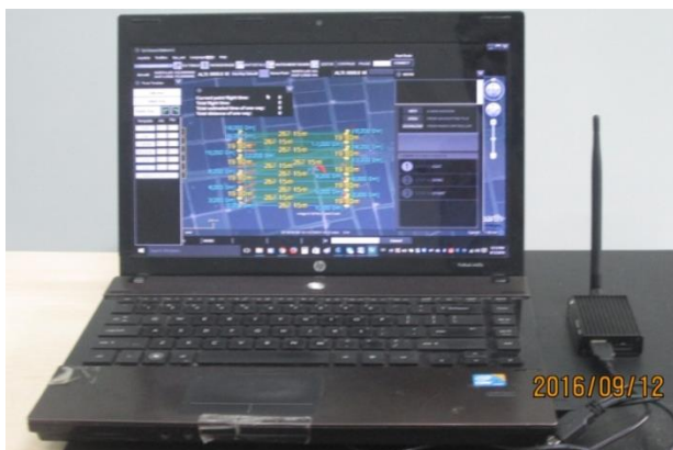
Figure 11: Ground station system using laptop as display
