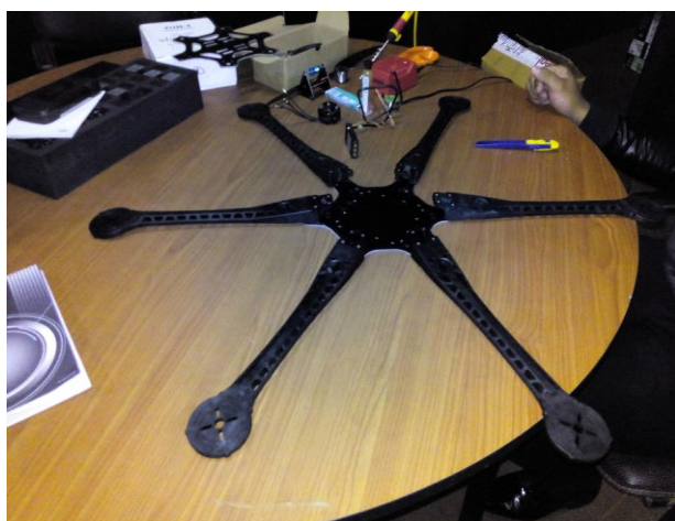
Figure 3: Hex copter frame assembled at NESAC
