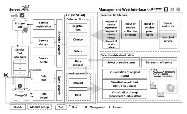
Figure 1. System architecture for the collection of public open data for mobile web visualization.
