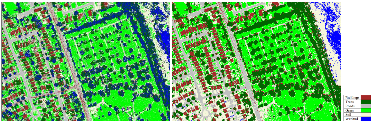
Figure 5. Classified images, from combined three-intensity images (left) and combined three-intensity images with DSM (right).
