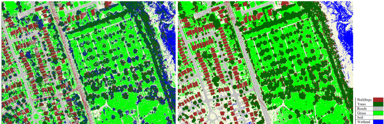
Figure 6. Classified images, from combined corrected intensity images (left) and combined corrected intensity images with DSM (right).
