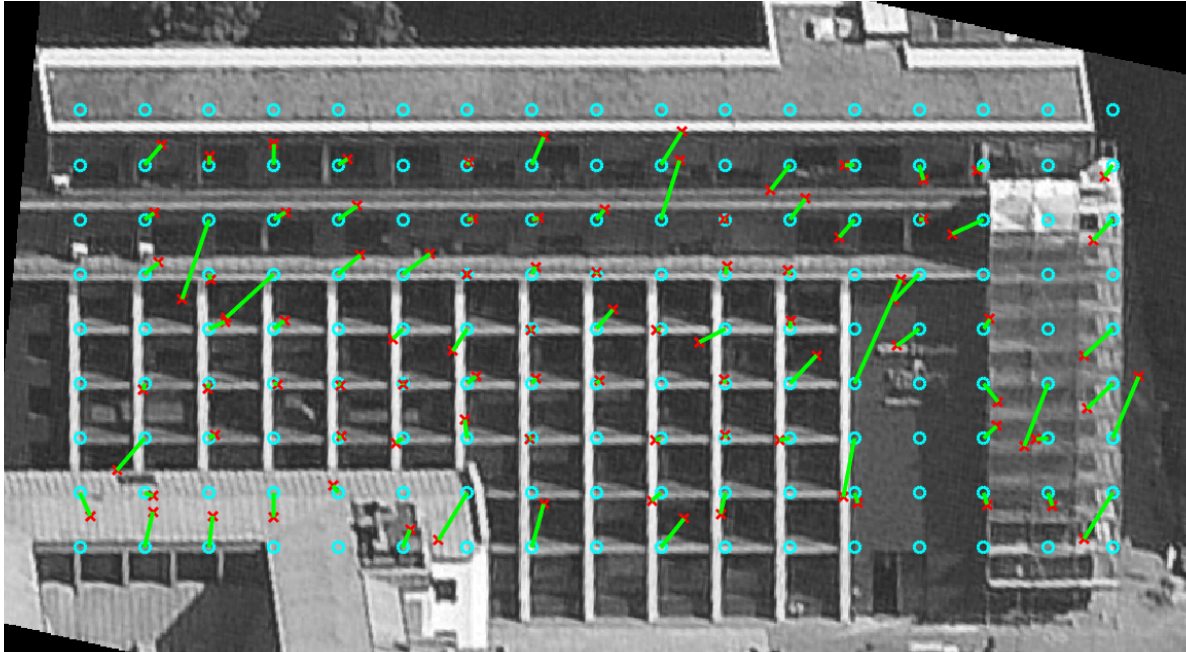
Figure 10: Matching result for case study 'Charlottenstrasse' with \alpha = 0.5 . Original PS positions are marked as red crosses. Lattice nodes are drawn as cyan circles. The matching is indicated by green lines.
