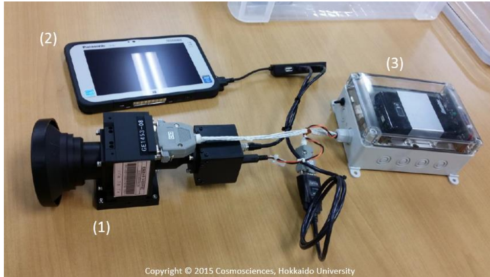
Figure 1. The (1) LCTF camera with the (2) controller and (3) power supply.
