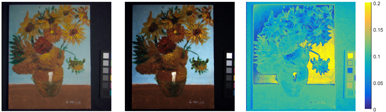
Figure 8. Original CAVE RGB (left), spectrally subsampled HSI (middle), residuals of the spectral response measured in absolute differences between intensities in the range [0 - 1] (right).
