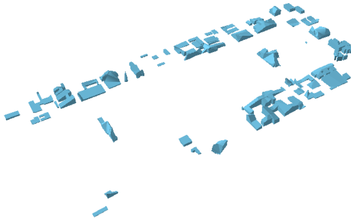
Figure 7. Extruded building polygons in three-dimensional space
