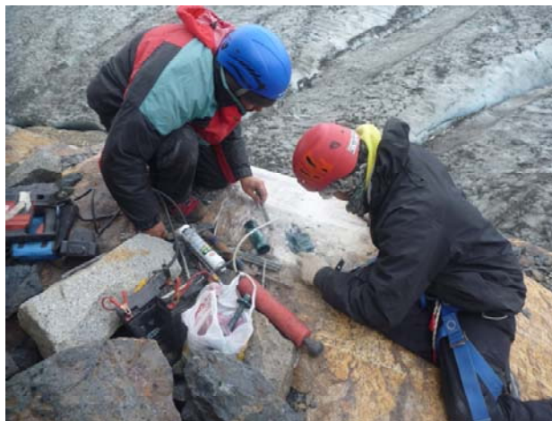
Figure 3. Camera cage installation at the South margin of Viedma Glacier.
