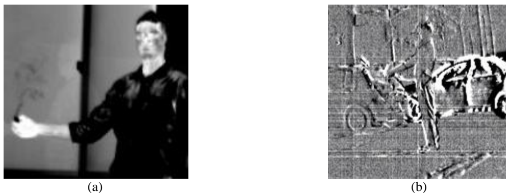
Figure 1: Examples for small gas plume detections with the FLIR GF320: (a) in an indoor environment with window as background, (b) in an outdoor environment using the differential enhancement mode
