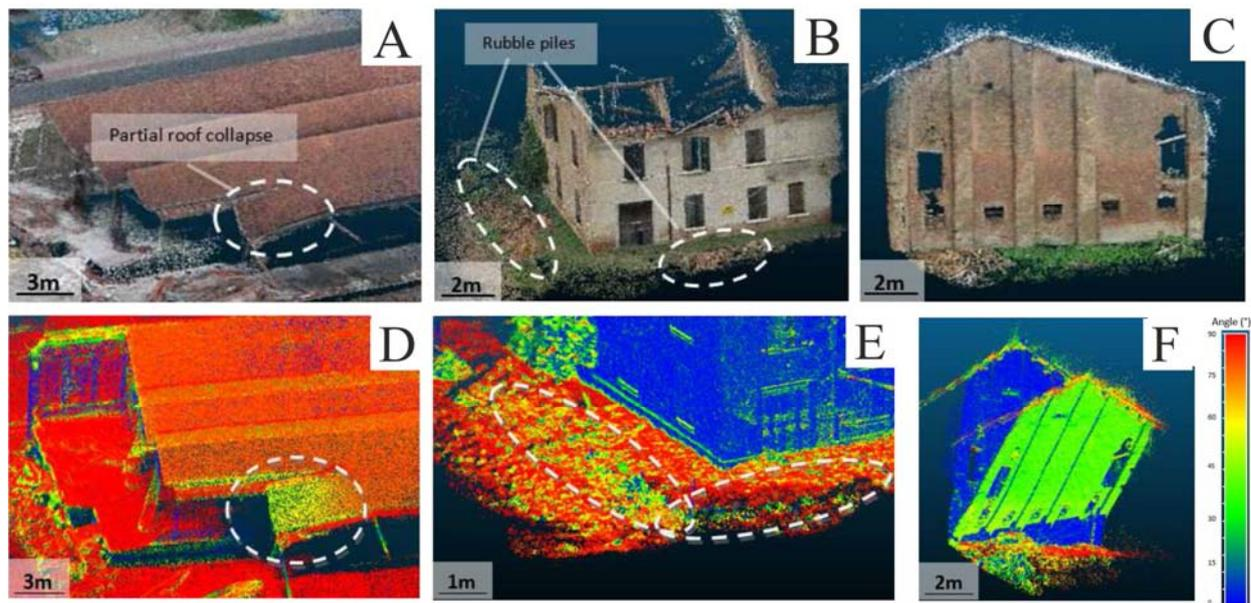
Figure 3: 3D point clouds of (A) a factory being demolished in Gronau (Germany, Aibot X6), and (B-C) buildings damaged by the 2012 earthquake near Bologna (Italy; pole-survey). Z-component of the normal of a local tangent plane calculated for adjacent points revealing geometric irregularities that correspond to different types of damage (D-F). See text for further details.
