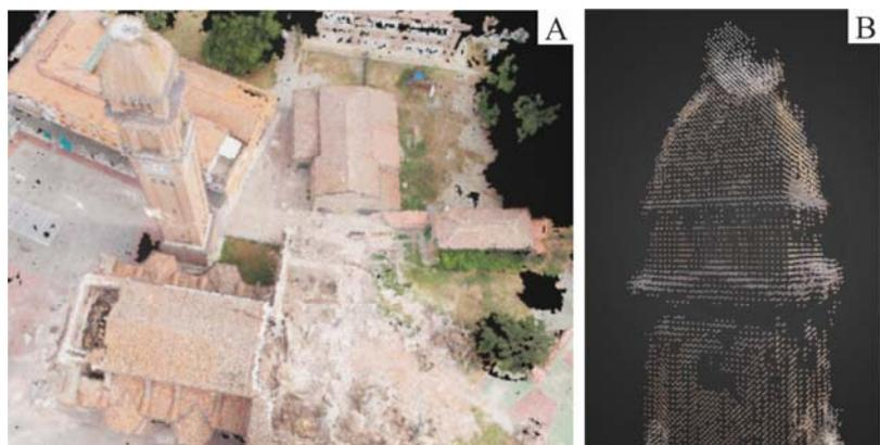
Figure 2: 3D point cloud of a damaged church in Mirabello (Italy)
