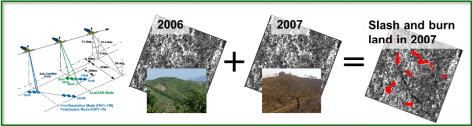
Figure 6: Change detection based on multi-temporal ALOS/PALSAR data analysis
