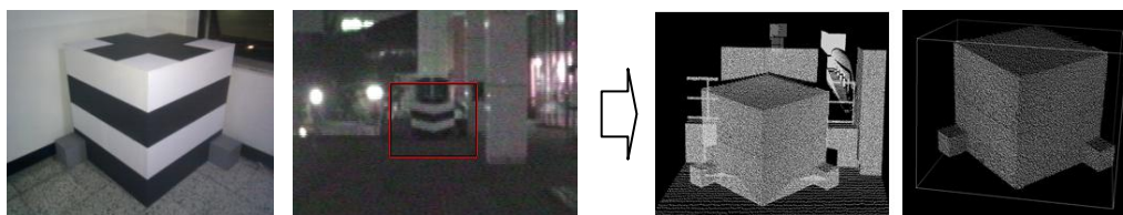
Figure 4. Miniature model and data acquisition area (left), Before/After outlier removal (right)
