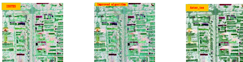
Fig.5. Comparison of retrieved emissivity and lib-acquired emissivity
