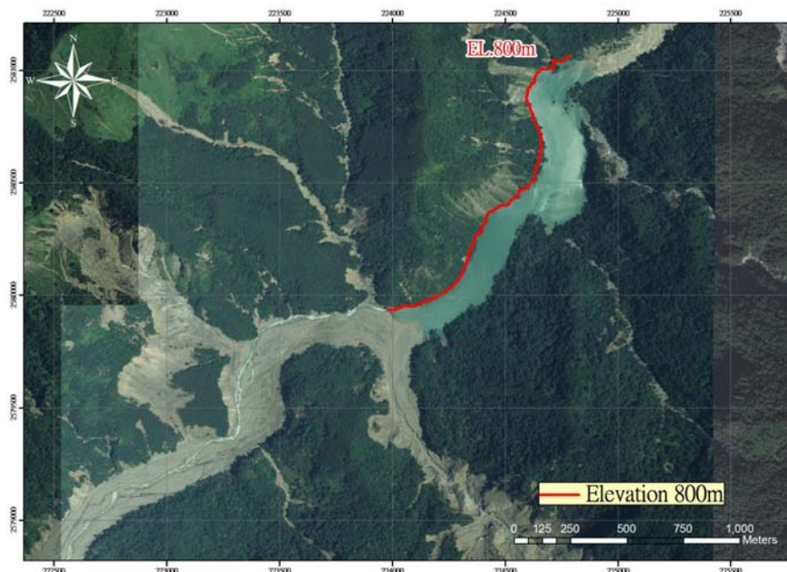
Figure 3. A contour with elevation of 800 m generated from the 5-m DTM which best fit the water-land boundary identified from the high-resolution aerial photograph.
