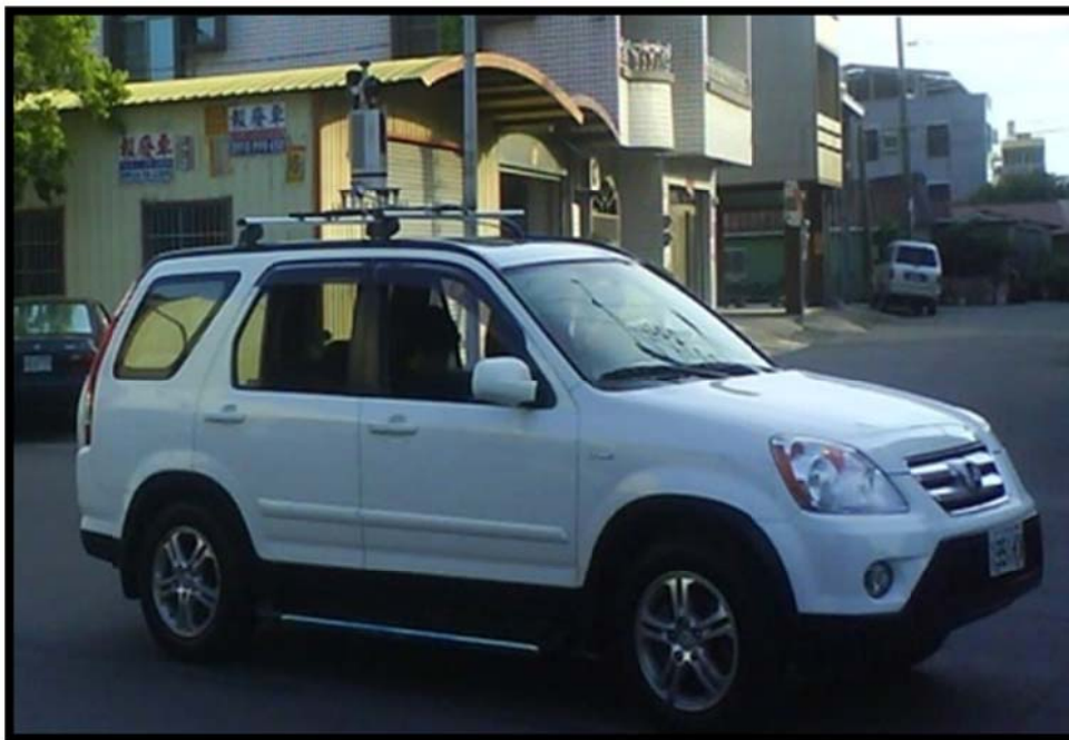
figure 3 RIEGL VZ400 surveying vehicle
