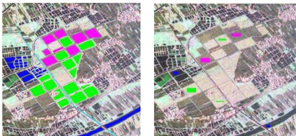
Figure 4. the ground truth data (left) and the chosen training pixels (right) in the test area, with pink (dry land), cyan (road), green (sugar cane) and blue (water body).
