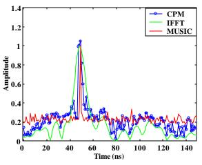
Fig. 2 IFFT, MUSIC and CPM response of signal plus noise at input at SNR -5.8 dB and M=30
