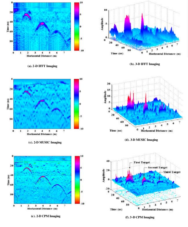
Fig. 5. Two Dimension and three Dimension images of IFFT, MUSIC and CPM response in linear scale at frequency bandwidth 400 MHz, M=10, L=50.
