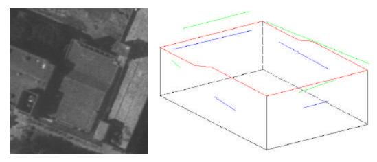
Fig. 11a and 11b the incorrect edges for outline due to occlusion and shadows
