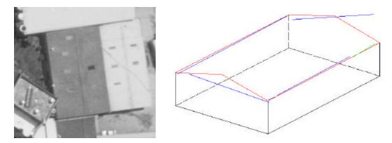
Fig. 10a and 10b the possible error lines of gable roof caused by Hough Transform
