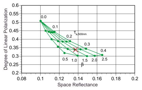
Figure2 Diagrams used by parameterized directional polarization - space reflectance in a single band; "×" represents a target area with observed reflectance and degree of linear polarization values over the desert (sand) area.
