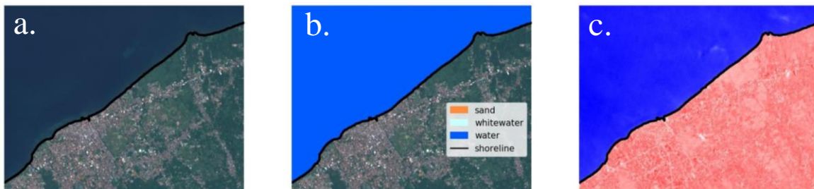
Figure 4. a) RGB image of certain study area; b) Output of image classification where each pixel has been labelled with one of three classes; c) Grayscale image of the MNDWI pixel values
