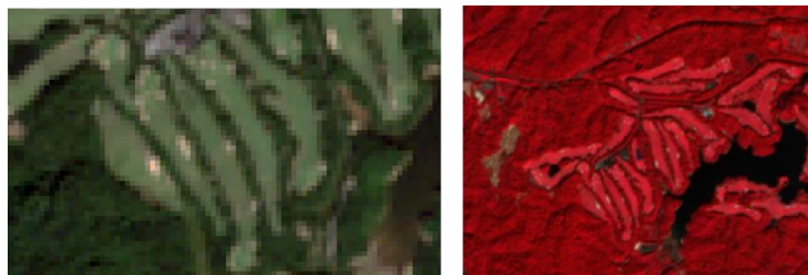
Figure 5. Sentinel-2 Image / Left: Zoomed in image of the course (RGB: B04, B03, B02), Right: Whole image of the course (False Color: B08, B04, B03)
