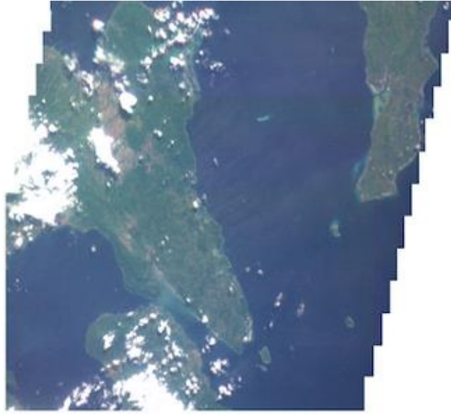
Figure 4: Diwata-2 SMI RGB mosaic after merging the equivalent of 13 unique image composites
