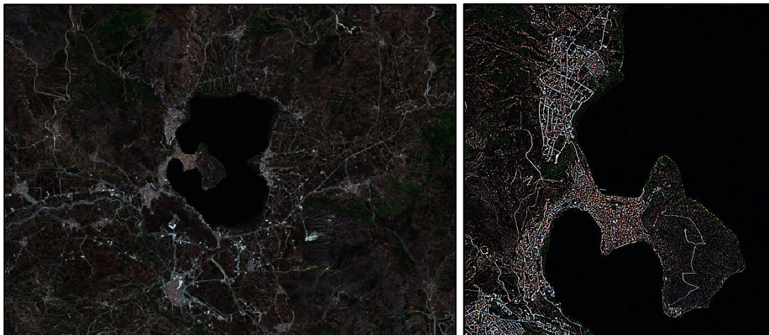
Figure 8. Sentinel-2 subsets of the study area after convolution filter for edge detection
