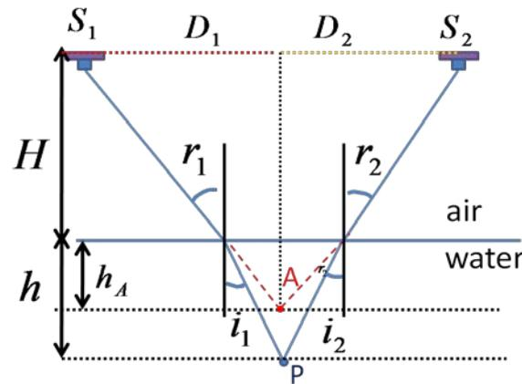
Fig. 2. Geomertry of two medium photogrammetry.
