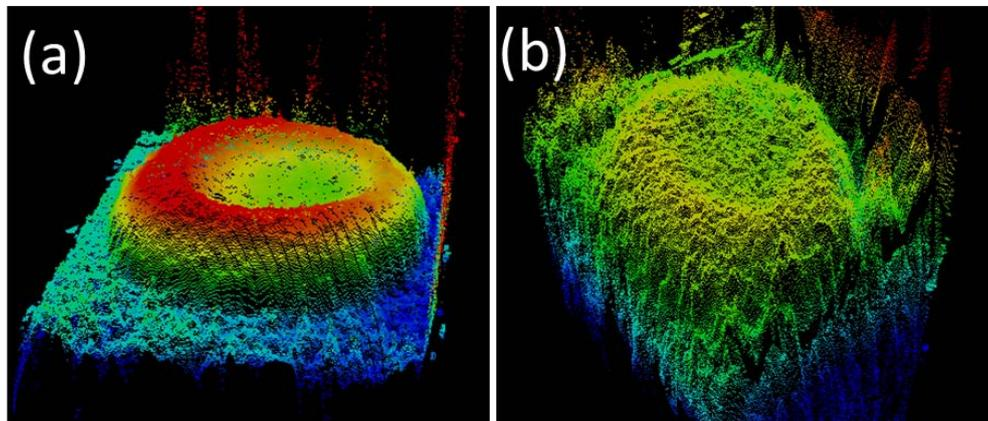
Fig. 6. The result of CLORAMA(a) Non-water DSM of test area(b) submerged DSM of test area.
