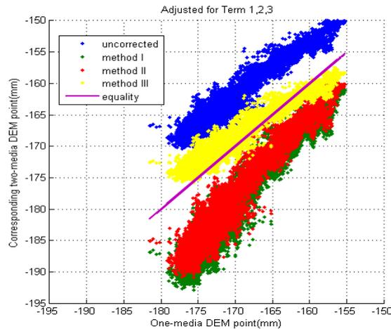
Fig. 10. The result of different correction method of test area. The blue line is apparent depth. Purple line is equality. And green line is method I resultant the red one is correct from method II. Green line is the correction result of method III
