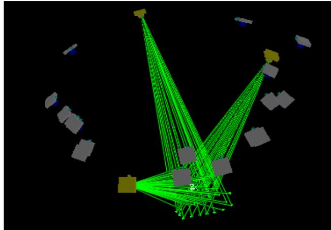
Fig. 5. The distribution and intersection of cameras locate in iWitness.
