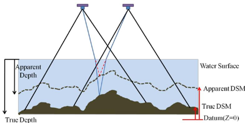
Fig. 1. The blue lines refract in the water and located in the true DSM. The red lines go straight into water and converge in apparent depth.
