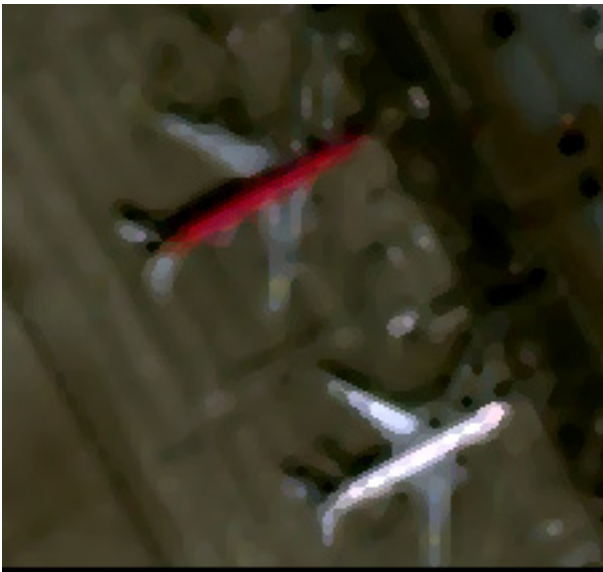
Figure 11. Median filtering image for two times enlarged image by using nearest neighbor method
