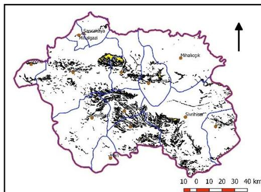
Figure 7 Results of suitable slope and aspect areas for the solar power plant installation.
