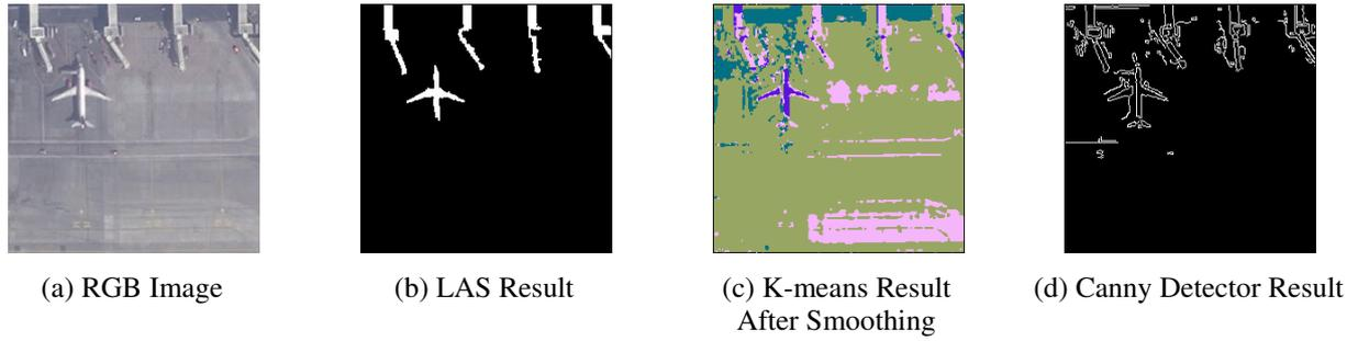
Figure 2. Comparison of LAS Segmentation Results
