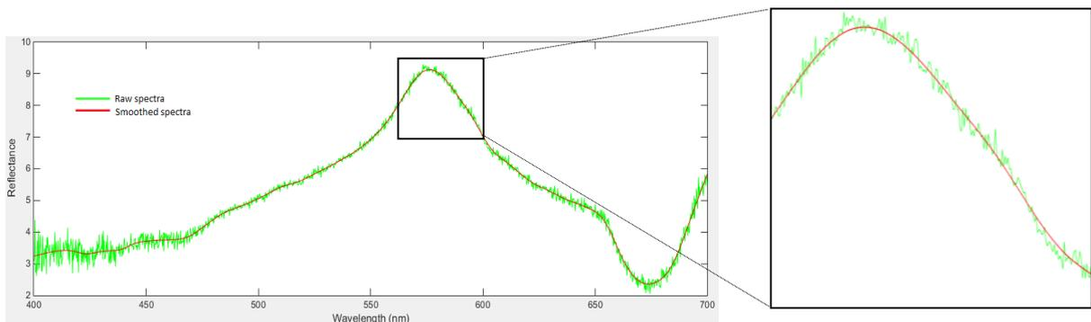
Figure 1. Result of smoothing a live coral spectrum using Savitzky-Golay algorithm (filter size = 50, degree of polynomial = 3); before smoothing (green); after smoothing (red)
