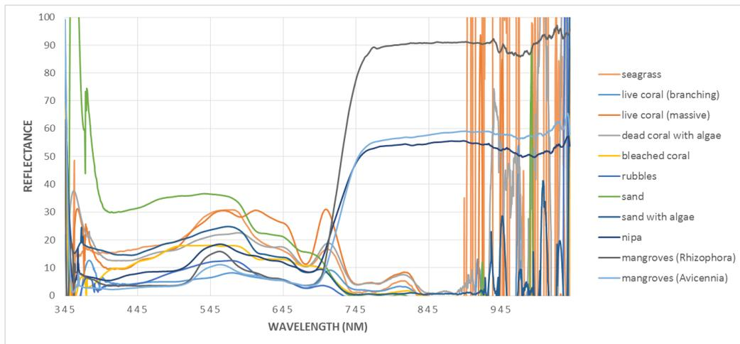
Figure 3. Sample filtered spectral reflectance curve patterns of various coastal resources over the wavelength range of 345 nm – 1035 nm
