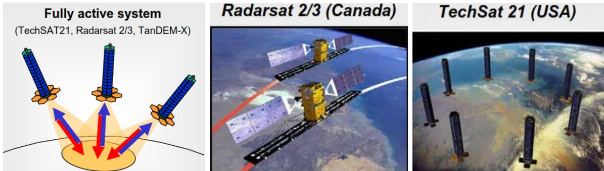
Figure 6: Space-borne SAR system in fully active configuration
